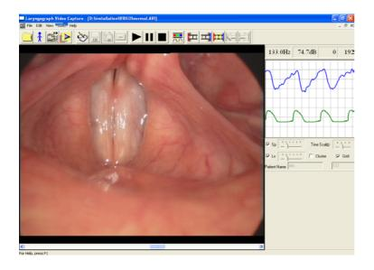
The Lx Video Capture system can be used with any continuous or stroboscopic light source, with rigid or flexible endoscopes and with a range of cameras.
