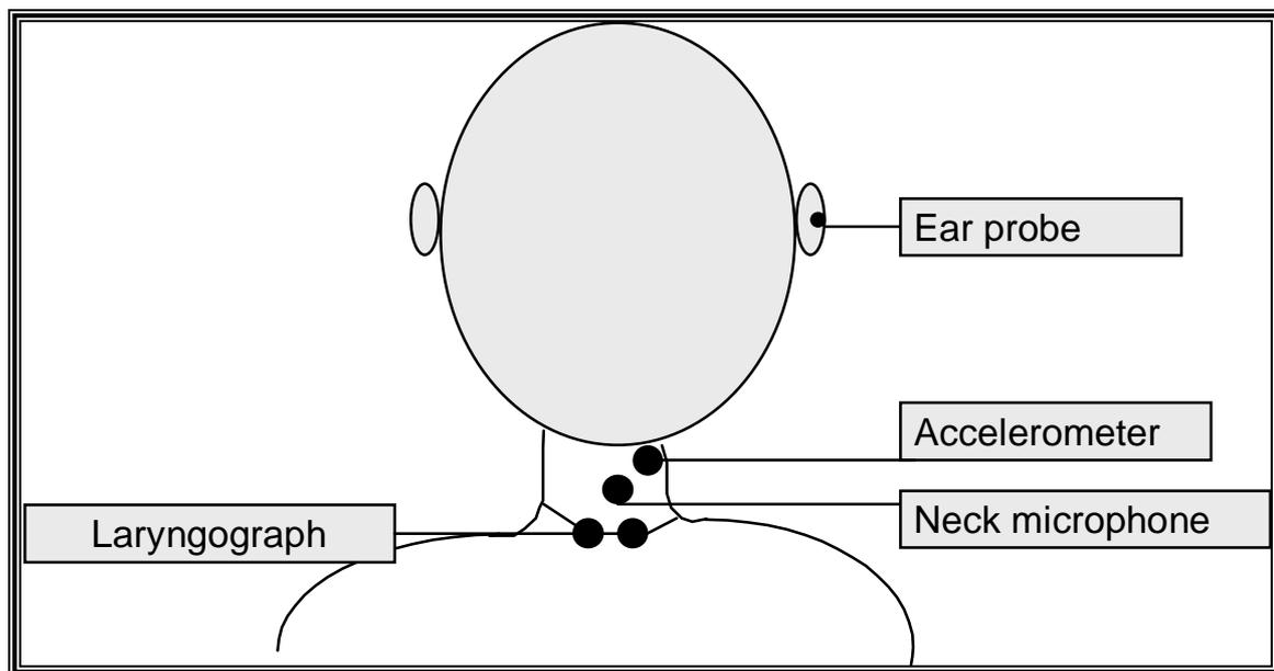
**Figure 5** *Sensor Placement*
